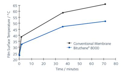
Comparsion of solar heat gain over time on exposed membrane samples.
