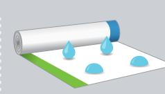
Preprufe Plus roll smooth, non-absorbent surface resists site contaminationon
